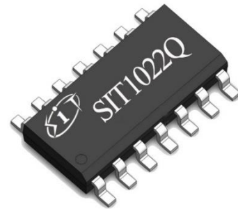
Fig 1. Provide environmentally friendly lead-free package
